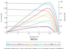
Excellent performance under weak light conditions: at an irradiation intensity of  $800W/m^2$  (AM 1.5, 25°C), 95.5% or higher of the STC efficiency(1000W/m<sup>2</sup>) is achieved.
