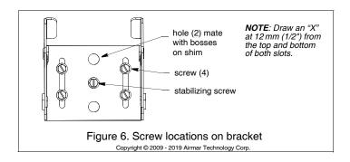
5. Using the vertical adjustment space in the bracket slots, slide the assembly up or down until the bottom inside corner of the transducer projections 0-3mm (0-1/8") below the bottom of the hull (Figure 1). When you are satisfied with the position of the transducer, tighten the four bracket screws. For clear access to the screws, remove the transducer assembly from the bracket (Figure 4). When reattaching, be sure to include the spacer.
