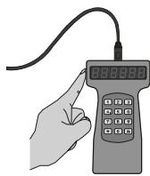
Turn off the CEU by pressing the side mounted switch to the "0" position.
